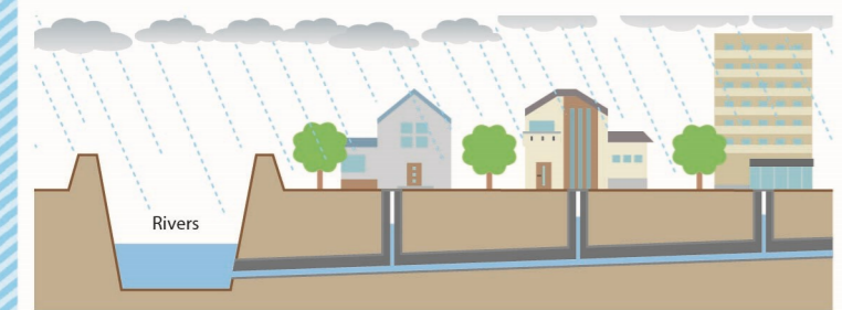
Rain that falls on residential areas and roads is drained into rivers through sewers and waterways.
