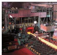
Steel sheets that are later used for juice cans, car bodies, and other purposes are produced at this hot rolling facility
